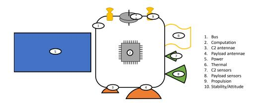
Figure 3: Component breakdown of common satellite subsystems for attach mechanism considerations
