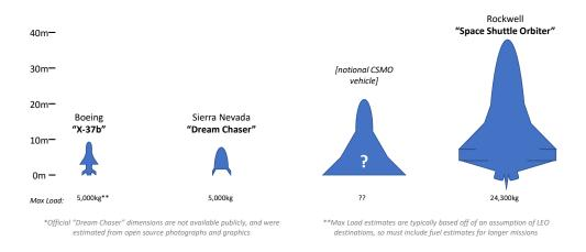
Figure 7: Comparison of three lifting-body spacecraft and notional scale of a CSMO vehicle
