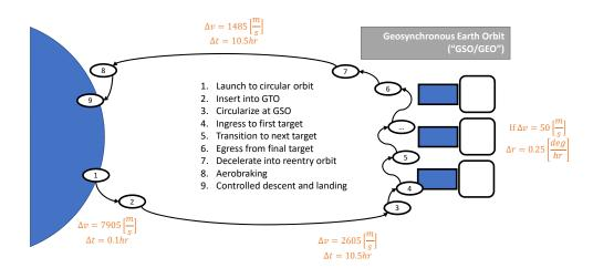
Figure 5: Mission sequence from steady-state through multi-target execution
