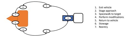
Figure 4: Staged ingress and egress encapsulates a careful, multi-step, coordinated activity
